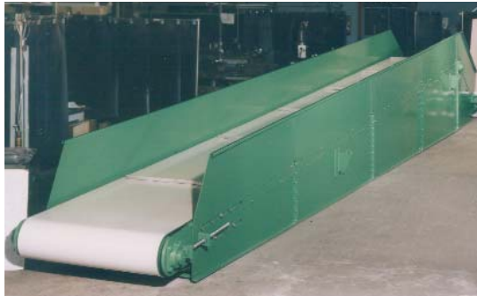
► Conveying belts for a recycling plant
