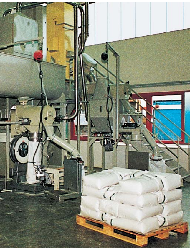
▲ Cascade sifter working acc. to the circulating air principle in a spice mill
